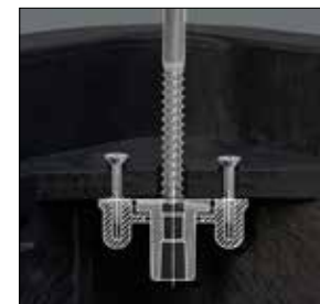
Non-Seizing Bolt System Allows Field Replacement
