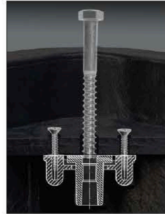
Non-Seizing Bolt System Allows Field Replacement
